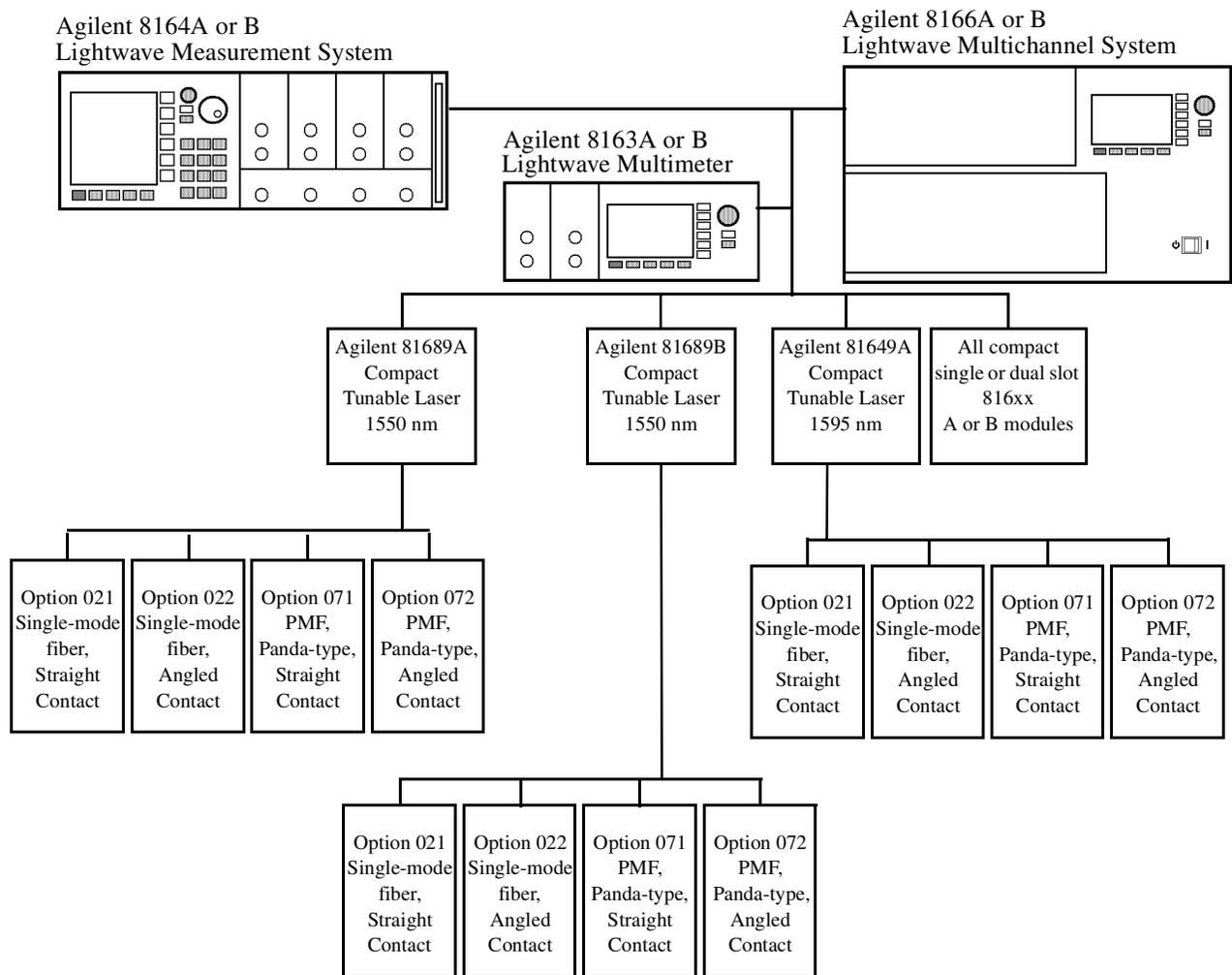
**Figure 8 Mainframes, Tunable Laser Modules, and Options**
