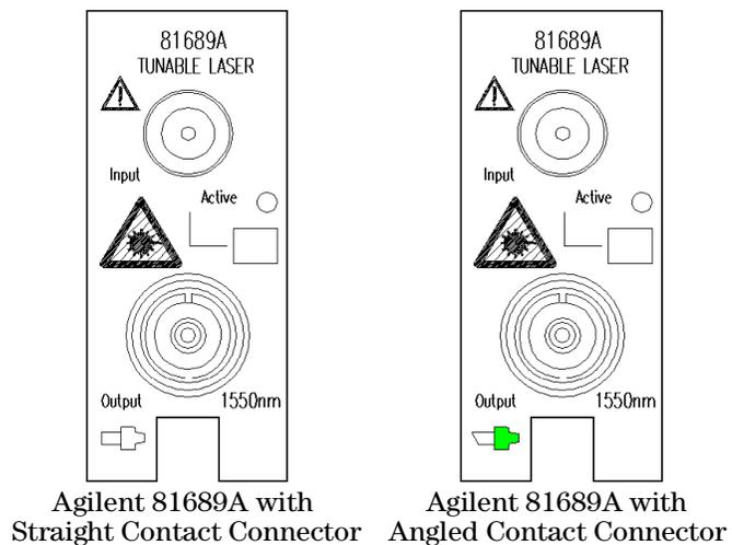
**Figure 3** Agilent 81689A Compact Tunable Laser Module
